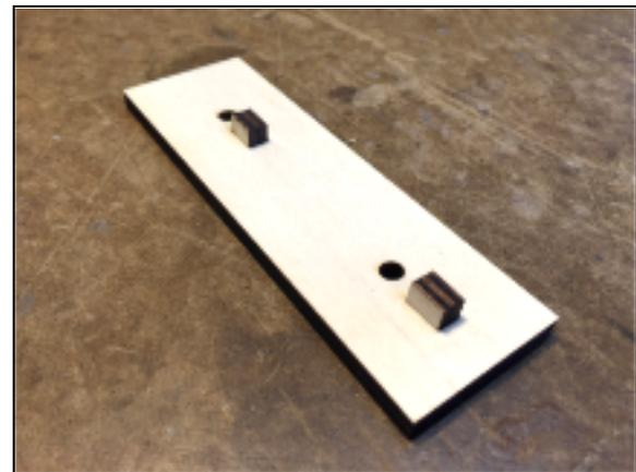
Now insert the rectangular connectors into the holes in the back brace. They should fit fairly snugly when inserted correctly, and part of the rectangular connectors should extend above the surface as shown.
