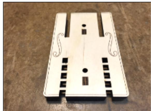
It is a good idea at this point to use some wood glue to secure the above pieces (back brace, rectangular connectors and faceplate) together securely.
