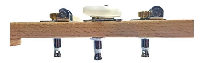
With the neck propped up, push your tuners through the holes making certain that the gear is on the "bottom" side of the tuner, aligned towards the tail-end of the neck, not the top. You've got one tuner hole on one side of the headstock and two on the other. So you'll have one tuner with a gear that is facing the tail end and two tuners doing the same on the other side. See what we mean in the photo below?
