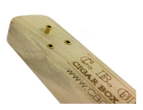
Push the six string ferrules into the holes in the tail end of the neck—3 in the front side and 3 in the back. They should press in fairly easily, but use your screwdriver handle to tap them into place if need be.
