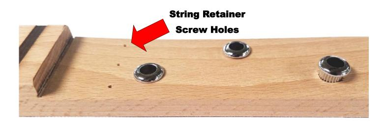
While you have the neck facing up, insert your three brass string retainer screws (**Part "E"**), one at a time, into the three holes that are in a line with one another on the headstock. They are located between the tuner bushings you just installed and groove that has been notched out for the nut.
