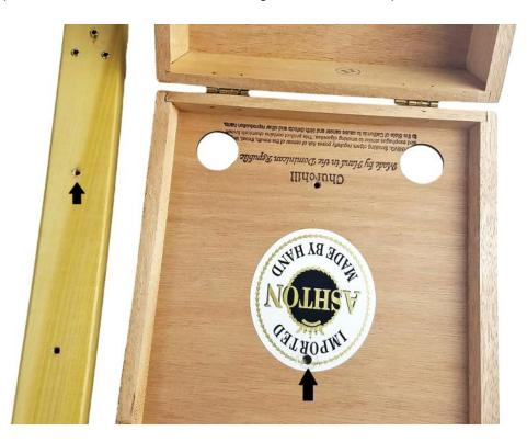
Open up your box and with the hinge side facing the headstock and your newly installed tuners, line up the holes in the box lid to the holes on the neck. Wielding your trusty Phillips head screwdriver, twist those two ¾" washer-head lath screws (**Part "F"**) into place.
